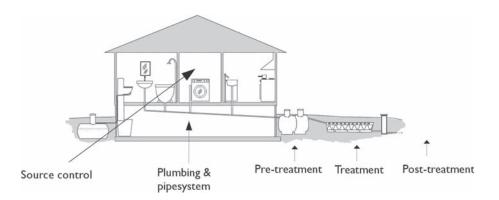
Figure 2. Components of a greywater management system.
