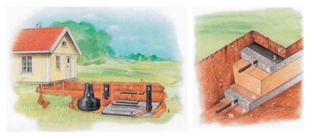
Figure 10. Design of a typical conventional sand filter system for onsite solution used in Sweden. Diagram to the left: 1. Flushing pipe connected to distribution pipe, 2. Collecting (measuring) well, 3. Discharge pipe, 4. Drainage pipe, 5. Distributing pipe, 6. Distributing (flow splitting) well, 7. Ventilation chimney, 8. Septic tank.
