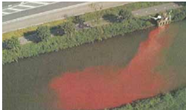
EFFLUENT PLUME FROM THE KATWOUDE STP, 10 MINUTES AFTER THE COMMENCEMENT OF THE DOSING OF A DYE (GHAUHARALI AND BOS, 2007)
